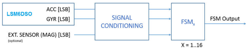
Figure 2. State machine in the LSM6DSO
